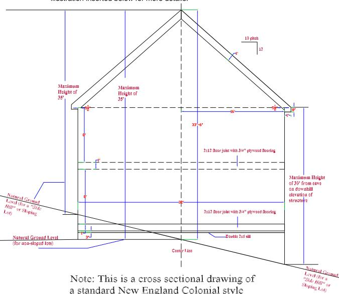
Note: This is a cross sectional drawing of a standard New England Colonial style home with a base width of 32'. Each floor has a thickness of 12" and a wall height of 8'. The roof has a 10 pitch for a total height from the "Natural Ground" to the ridge of 33'- 6".
